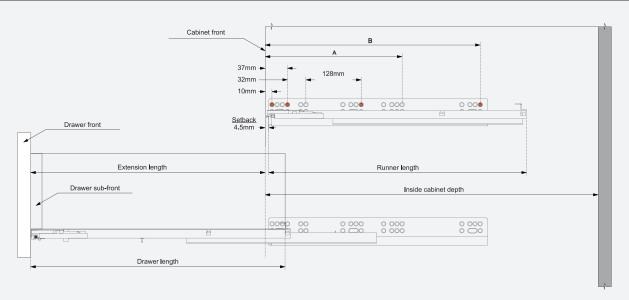
Note: The orange dots show the locations where fixing screws should be installed to achieve the specified load ratings
