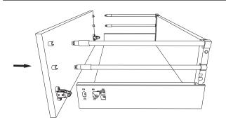
Assemble front panel on to the drawer.
