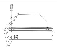
Tighten selftapping screws to fix bottom.
